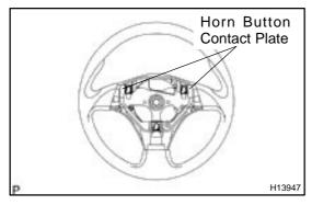
• Check the deformation of the horn button contact plate of the steering wheel.
